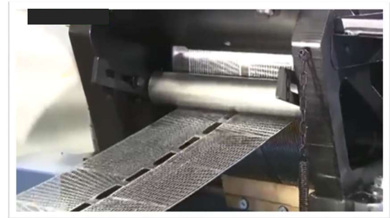
Grid casting from a caster drum
